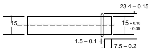
Fig. 10. Pipe end for "O"-ring connection
